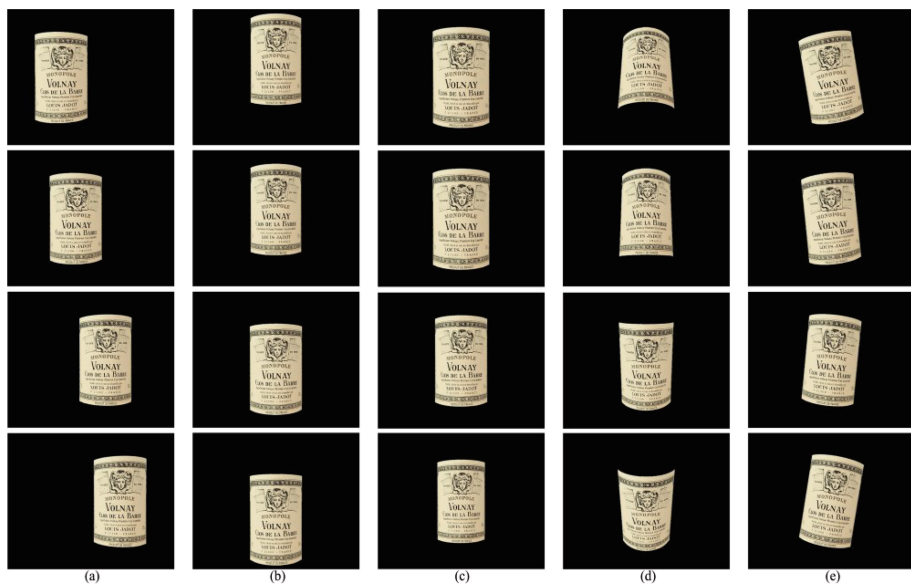
Fig. 6. Visually realistic ( 640 \times 480 ) images synthesized upon a virtual (invisible) wine bottle which is translated between (a) x = -40 mm and x = 40 mm, (b) y = -20 mm and y = 20 mm, and (c) z = 230 mm and z = 270 mm and rotated between (d) -30^\circ and 30^\circ w.r.t. the x-axis, and (e) -10^\circ and 10^\circ w.r.t. the z-axis.
