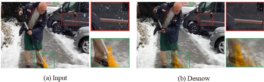
Fig. 1. The performance of S2VD [6] on a real snowy video. Red box indicates area where snowflakes have not been completely removed and green box indicates area where artifacts appear.
