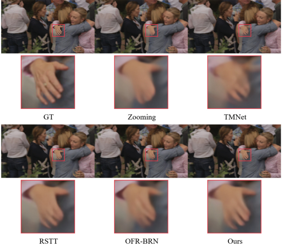
Fig. 5. Visual comparisons of different STVSR methods on Vimeo dataset. Parts of the areas are zoomed in and framed with red boxes to facilitate comparison. (Color figure online)
