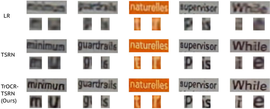
Fig. 5. Visual Comparison: LR input, SR output from the original TSRN [28] and SR output from TSRN trained with our TrOCR loss.
