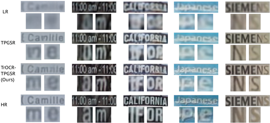
Fig. 6. Visual Comparison: LR input, TPGSR output after Stage 1 (TPGSR only), TrOCR-TPGSR output after Stage 3 (with TrOCR loss), and HR ground truth.
