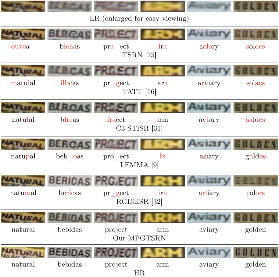
Fig. 7. Examples of super-resolution results obtained by different methods. LR denotes the input low-resolution image. HR denotes the ground-truth high-resolution image. Text under an image is the recognition result, in which the red characters are incorrectly recognized ones and ‘_’ denotes a missing character. (Color figure online)
