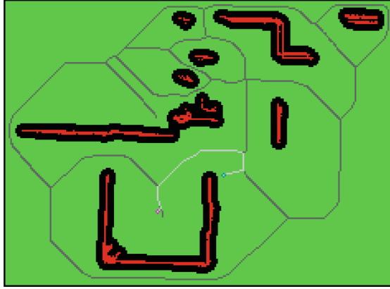
Fig. 5. Sample path generated from the medial axis algorithm. The path (light gray) connects the current (magenta) and target (dark blue) coordinates through the medial axis (dark gray), entirely within the traversable region (green) and maximizing distance from obstacles (red). Black denotes lethal cost. (Color figure online)
