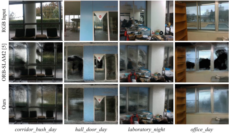
Fig. 8. Comparison of dense reconstruction for glass surfaces between our proposed ORB-SLAM2-GSD and ORB-SLAM2 [5] on our GS RGB-D dataset.
