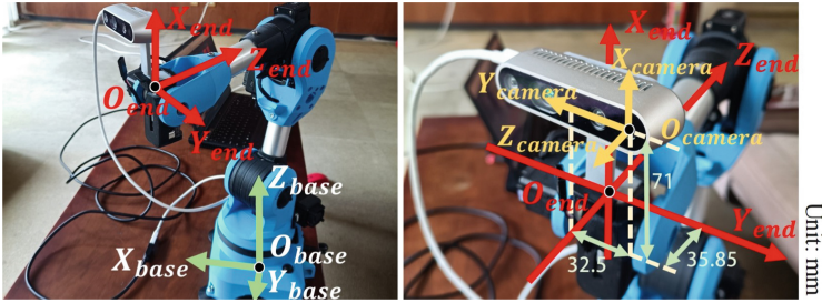
Fig. 6. Our camera-robot arm system. Left: The definition of coordinate systems for the robot arm’s base (green) and end (red). Right: The relationship between the coordinate system of the robot arm’s end (red) and the camera (yellow). (Color figure online)
