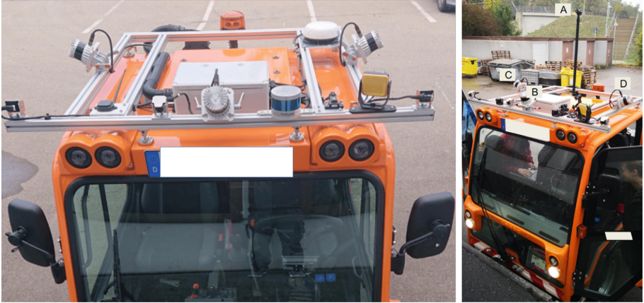
Fig. 2. Sensor setup on the data collection vehicle. Ouster lidar sensors are positioned at the front, right, and left (B, C, D). The 360° camera is mounted at A.
