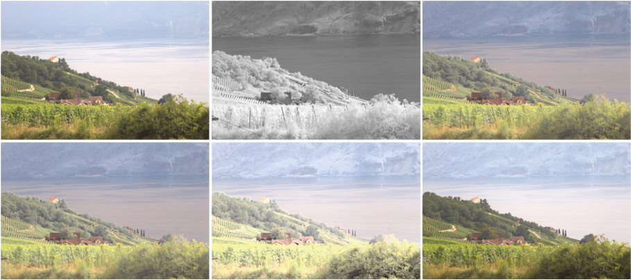
Fig. 6. Fusion results by different methods. Top: RGB image, NIR image, DenseFuse [15]. Bottom: DIF-Net [10], NestFuse [16], LDINet. LDINet generates a natural-looking fusion image with fine details while keeping the original color tone.
