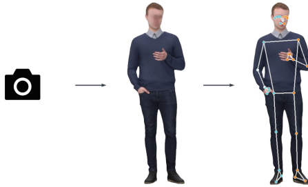
Fig. 4. Camera feed takes the human body as input and pose landmarker estimates the body pose using human landmark points
