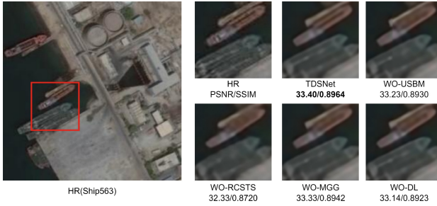
Fig. 5. Ablation results figure. From top to bottom, left to right: original high-resolution image, results from our proposed network, results without USBM, results without RCSTS, results without MGG, and results without dual loss.
