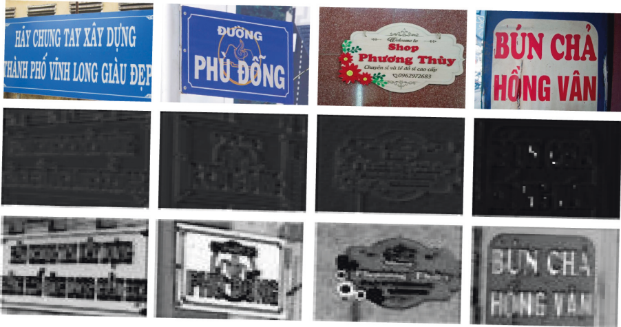
Fig. 5. Visualization of feature maps after the first stage of Resnet, where the top row includes original images, the middle row presents the feature maps when EIEM was not used, and the bottom row presents the feature maps when EIEM was used. In addition, to make the images clear, we have standardized the scale changes
