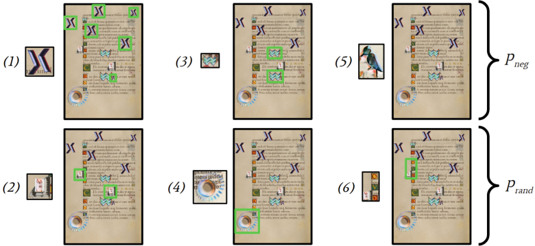
Fig. 4. Possible training pairs for a given target image. Pairs (1) through (4) showcase standard pairing for the 4 unique queries present in the target. Pairs (5) and (6) showcase respectively an example pair for the negative query sampling and random patch cropping . Green boxes represent the output objective for each pair.
