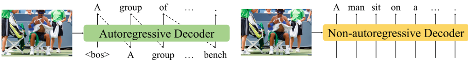
Fig. 1. The autoregressive image captioning model generates words one by one, while the non-autoregressive model generates words in parallel, which can greatly improve the inference speed of the model.
