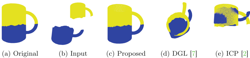
Fig. 1. The proposed method reconstructs accurately the mug by assembling the two parts, where the other approaches fail drastically in this case.
