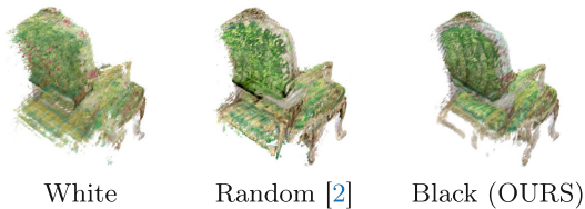
Fig. 6. Effect of Black Blending: Black blending clearly outperforms other methods, resulting in cleaner outcomes. It notably sharpens object boundaries and allows for a more accurate estimation of object shapes.
