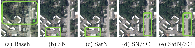
Fig. 7. RGB output from all NeRF variants. BaseN: Base NeRF, SN: S-NeRF, SatN: Sat-NeRF, SC: Solar Correction
