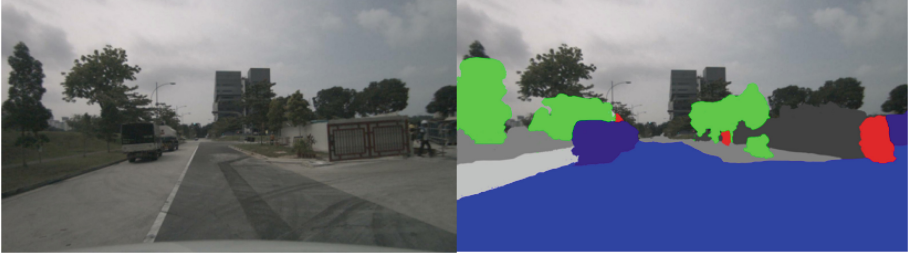
Fig. 3. The full semantic segmentation ground truth for camera images constructed according to the method in this article, the semantic free part in the figure is both the part that exceeds the occupied grid range.
