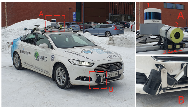
Fig. 2. The research vehicle ARVO used for data collection. The long-range sensors shown in box A are 1. LiDAR, 2. RGB camera in a weatherproof housing and 3. thermal cameras. The road weather sensor is shown in box B.
