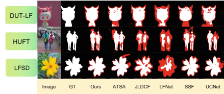
Fig. 7. Qualitative Comparison on three datasets. The difference maps between the visual results of various methods and the ground truth are displayed. Red pixels indicate pixels where the predicted results do not align with the ground truth. (Color figure online)
