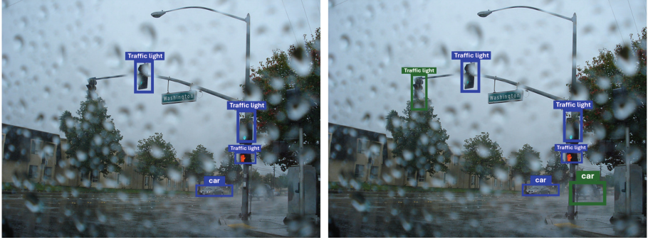
Fig. 1. An example of qualitative results using YOLOv8 on the COCO-2017 dataset: (left) object detection using an out-of-the-box YoloV8 model, where YOLOv8 fails to detect the Car in the bottom-right corner and one of the Traffic Lights in the upper left quadrant. (right) YOLOv8 enhanced with LLaMA 2 pt , where our integrated approach accurately finds these missed objects. The green boxes in the right image highlight the correctly detected objects which were missed by the standard YOLOv8 model. (Color figure online)
