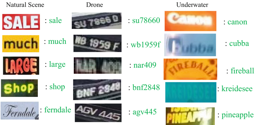
Fig. 5. Proposed model’s recognition results on multiple domains. Characters in green represent the correct predictions, whereas characters in red represent the wrong predictions.
