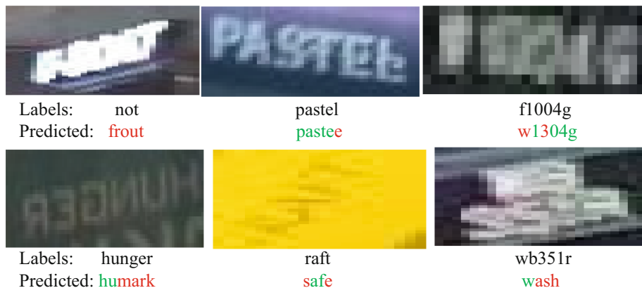
Fig. 6. Failure cases of the proposed model. Characters in green represent the correct predictions, whereas characters in red represent the wrong predictions.
