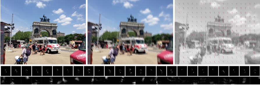
Fig. 3. Example of adaptive decomposition of Dense motion kernel Map. The images in the top row from left to right are, sharp image, synthetic blurry image, and visualized kernel map. The following two lines are the decomposed kernel basis and corresponding mixing coefficients respectively.
