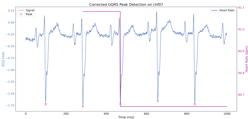
Fig. 3. Corrected GQRS R-Peak Detection used to extract R Peaks and RR Intervals
