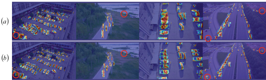
Fig. 6. The heat maps of (a)YOLOv8; (b) BiPA-Net on the Visdrone2019 dataset.
