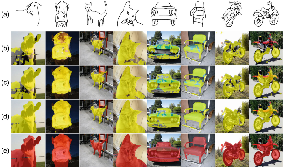
Fig. 5. Result of Instance-level Segmentation on SketchySeg. (a) Input sketch for sketch2seg model. (b) Segmentation results of DDPM-Seg. (c) Segmentation results of sketch2seg + text. (d) Segmentation results of sketch2seg + sketch. (e) Ground-truth segmentation map
