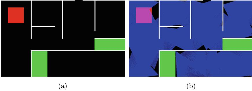
**Fig. 11.** Plan image of (a) Office space with user-specified constraints (b) Coverage results of m-EGGV algorithm
