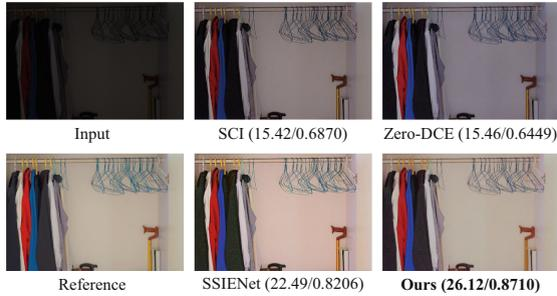
**Fig. 1.** Qualitative and quantitative (PSNR/SSIM) comparisons of state-of-the-art unsupervised methods, including SCI [33], Zero-DCE [9], SSIENet [43], and our approach. Our method preserves more consistent information than the others.
