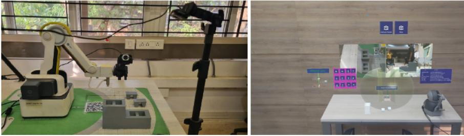
**Fig. 2.** MR based Robot Teleoperation
