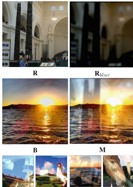
Fig. 3. This figure illustrates the process of synthesizing images. Here, \mathbf{R} represents the reflection image that undergoes Gaussian blurring to yield \mathbf{R}_{blur} , a blurred version of the original reflection. \mathbf{B} refers to the background image, and \mathbf{M} signifies the final synthesized image, produced by combining \mathbf{B} and \mathbf{R}_{blur} . Additionally, four examples of synthesized reflection images are presented at the bottom of the figure.
