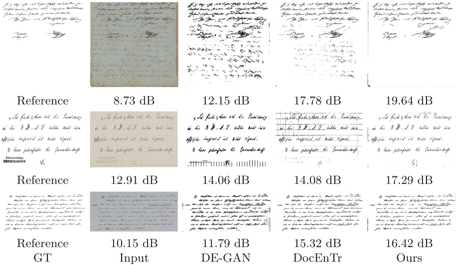
Fig. 3. Qualitative comparison of document binarization on DIBCO'19[29] dataset, the Figure is best readable in 300% zoom.
