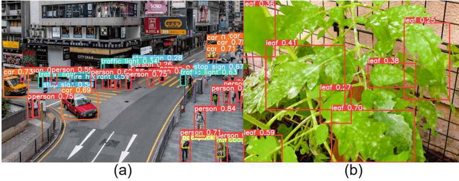
Fig. 1. In the images we can see predictions made by two different YOLOv8 [25] models in the form of rectangular boxes called bounding boxes; each box is assigned a class along with a confidence score by the model. (a) A trained YOLOv8 [25] on COCO 2017 dataset for multiple objects, (b) A YOLOv8 trained on Plant-Doc [22] Object Detection dataset detect leaves.
