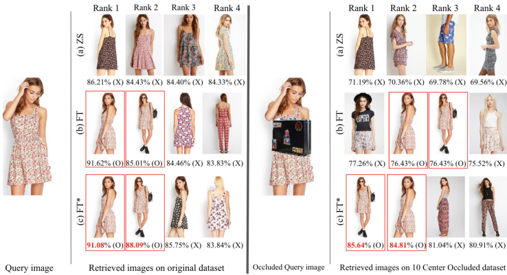
Fig. 6. Retrieved images with non-occluded (left) and occluded (right) query image. Each row indicates the top 4 ranked retrieved images and their confidence scores for each model—(a) ZS (zero-shot), (b) FT (fine-tuned on non-occluded images), and (c) FT* (fine-tuned on occluded images). Correctly retrieved images are represented with red edges.
