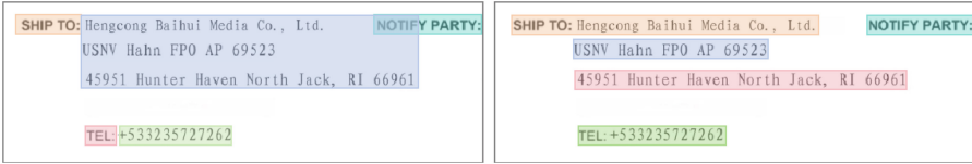
Fig. 2. Illustration of span detection and text aggregation issue. Text bounding boxes are marked in different colours for differentiation. Left: entity-level OCR results used by previous methods. Right: outputs of real-world OCR engines, only line-level bounding boxes are provided, and contents of two entities may be merged.
