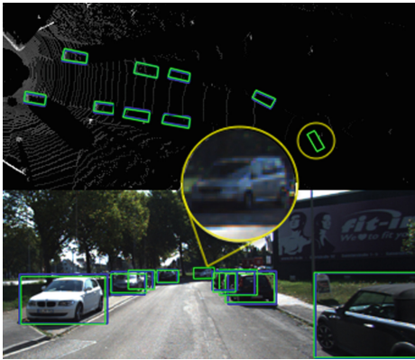
Fig. 6. Sample from the KITTI dataset illustrating the capability of our network to accurately detect an object despite incorrect annotation. The green bounding box indicates true positive detection, while the blue bounding box represents ground truth.
