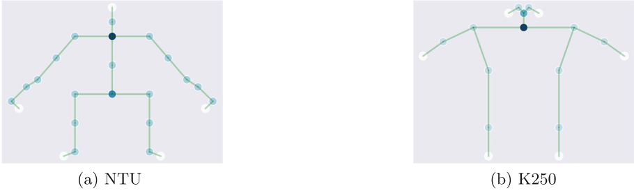
Fig. 10. The degree of joint nodes for each type of skeleton graph is represented by color intensity: the darker the joint node, the higher its degree.
